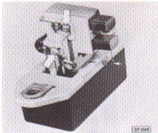
Fig. 1 Checking voltage regulator/carbon brushes
