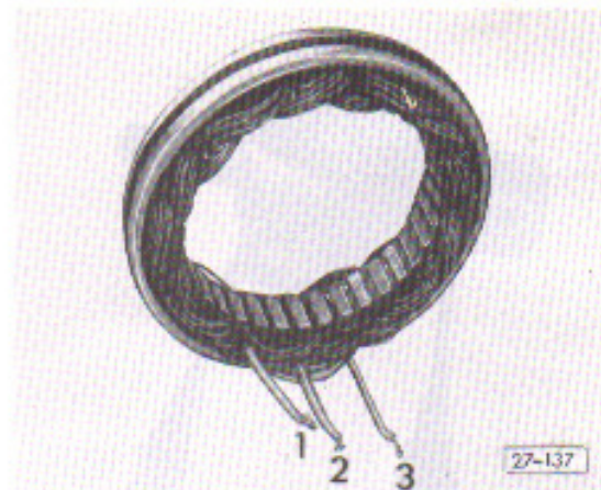
Fig. 11 Checking stator/open circuit
