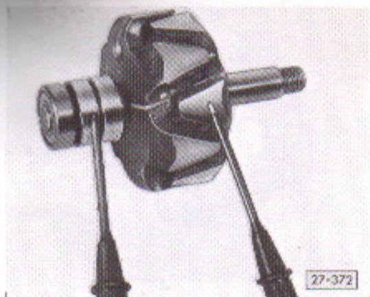
Fig. 13 Checking rotor/earth short
